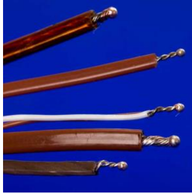
Pre-cut Validation Thermocouples
